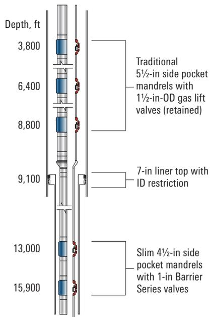
*Schlumberger installed two 1-in Barrier Series gas lift valves in slim 4 1/2-in side pocket mandrels that had a special 6-in drift OD suitable for the 32-lbm/ft, 7-in liner. As a result, the gas injection depth was extended from 9,095 ft (just above the liner top) to 15,900 ft, where the well deviation is 69°, optimizing drawdown and production.*
