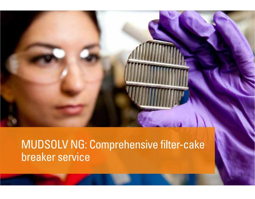
A properly formulated and carefully maintained reservoir drill-in fluid (RDF) deposits a dense and ultra-low permeability filter-cake on the surface of the formation, preventing significant invasion of reservoir-damaging fluid and solids. Depending on the completion type installed, if the filter-cake is not uniformly and completely removed it may subsequently impair well productivity or injectivity.
