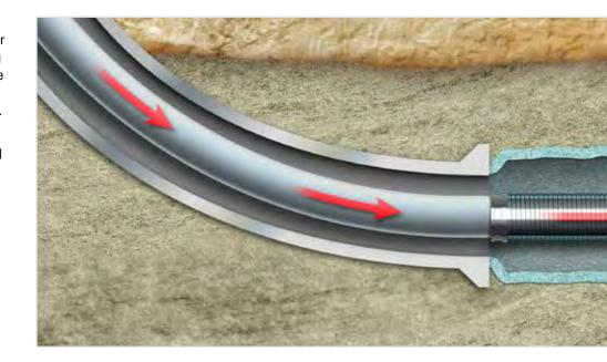
The MUDSOLV NG approach allows slow-reacting (non aggressive) treatments to be carried to all areas of the filter cake in the wellbore (as during simultaneous gravel packing and cleanup). Uniformity of cleanup is improved, and the pressure required to flow into the completion along its entire length is reduced.
