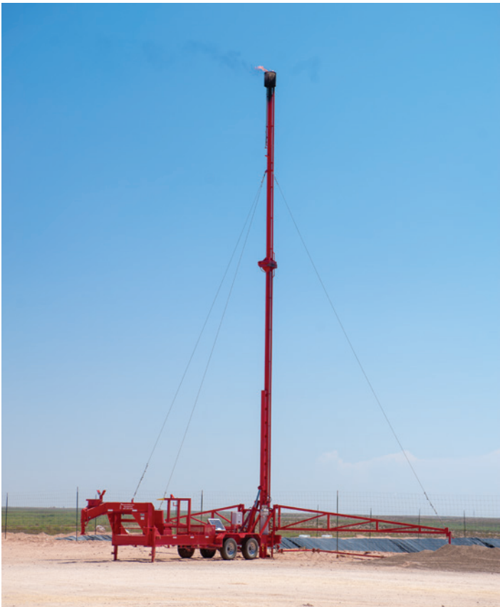
Flare systems are available in 3-, 4- or 6-in-diameter stacks with multiple heights.
