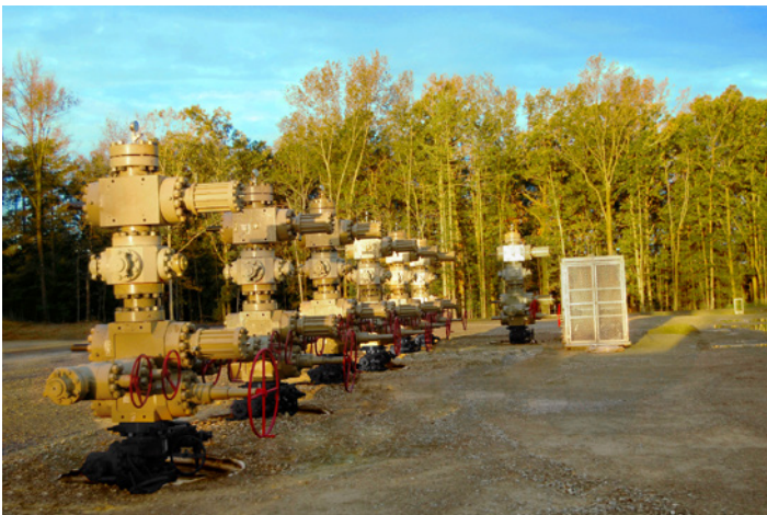
These Cameron composite fracture trees are operating in a seven-well pad in the Fayetteville Shale.
