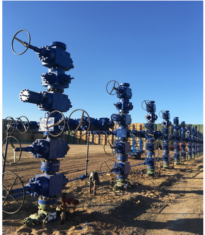
Cameron gate valves in frac trees and manifolds can reliably flow and control high-pressure, high-volume, erosive, corrosive, and sometimes sour fracturing and flowback fluids for days.
