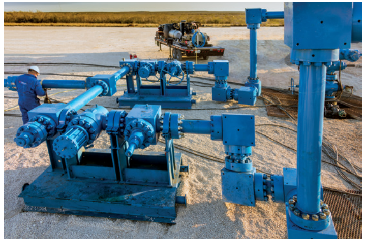
Monoline technology presents a safer, faster, cleaner alternative to conventional frac iron on multiwell pads, changing the way proppant and fracturing fluid are delivered from the pump spread to the wellbore.
