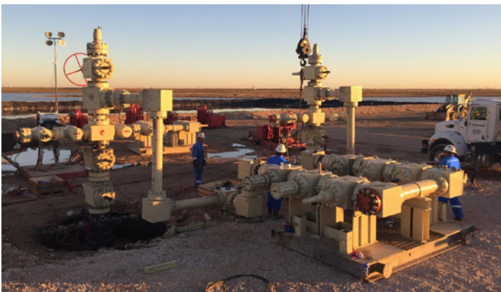
Monoline technology offers a larger diameter for increased flow rate, mitigating erosive fluid velocities; a streamlined design to facilitate installation and reduce the bends in the flow path; and a safer connection that reduces failure points.
