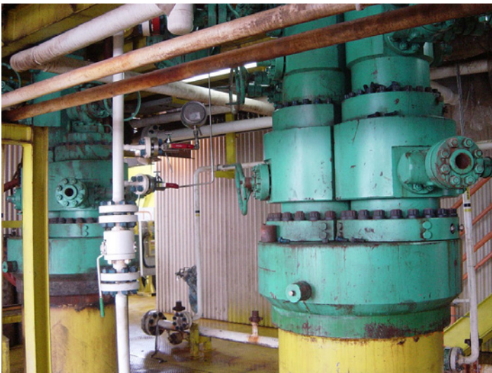
The CSW wellhead system enables multiple wells to be drilled from a single platform slot.
