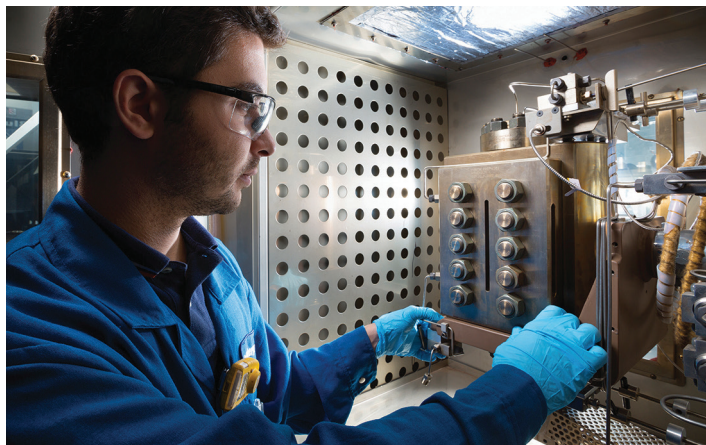
PVT analysis. The Schlumberger mercury-free PVT system, manufactured by the Schlumberger DBR Technology Center in Edmonton, has delivered thousands of PVT studies—from lean condensates to heavy oils.
