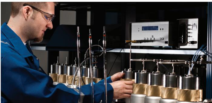
Core analysis, such as measurement of the electrical properties of formation samples, provides important information to tune log interpretations.
