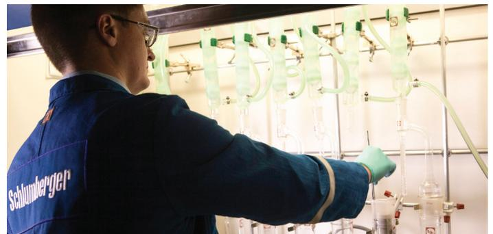
Careful core cleaning techniques are performed using a Dean-Stark apparatus to determine water content.
