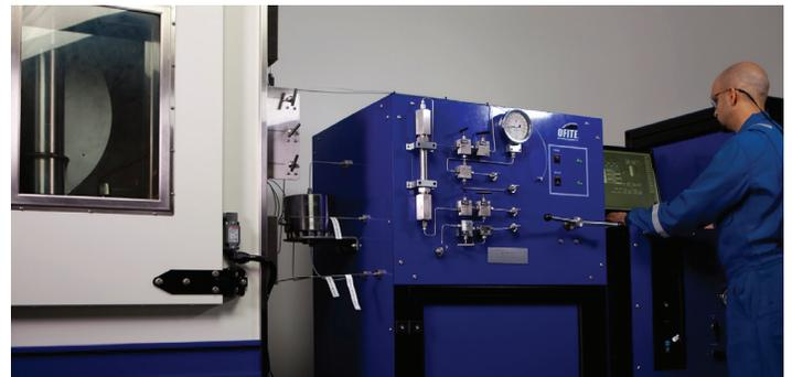
Coreflood studies help evaluate waterflood and EOR processes and are used to assess formation damage caused by a variety of sources.
